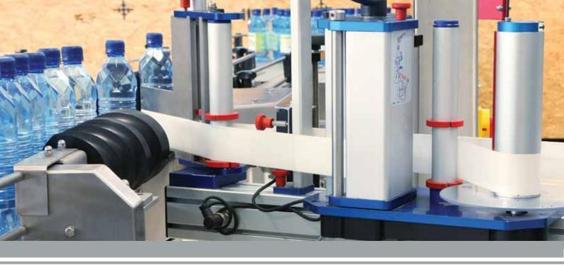
**Wing Eco Labellers** are specifically designed and customisable to customer requirements and are available in a number of configurations including single or twin labelling heads.
